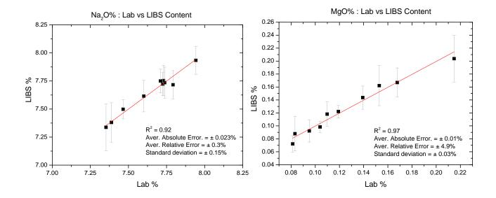
Calibration results between provided laboratory data and LIBS analysis, show proper correlation, thus possibility of on-line, real time LIBS analysis is definite.
