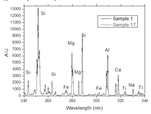
As can be seen from UV range spectra, well defined lines of: Si, Ti, Al, Ca, Fe, Mg and Na can be clearly detected. This chart shows quality comparison between sample 1(black) and sample 17 (red). As can be seen, while LIBS Si, Al and Na lines are higher in sample 1, Mg, Fe, Ti and Ca lines are higher in sample 17, as it should be, according to attached chemical data.
