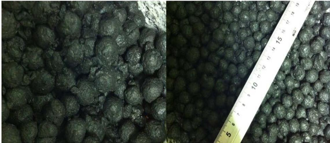
Picture 1. Unprocessed iron ore pellet.
