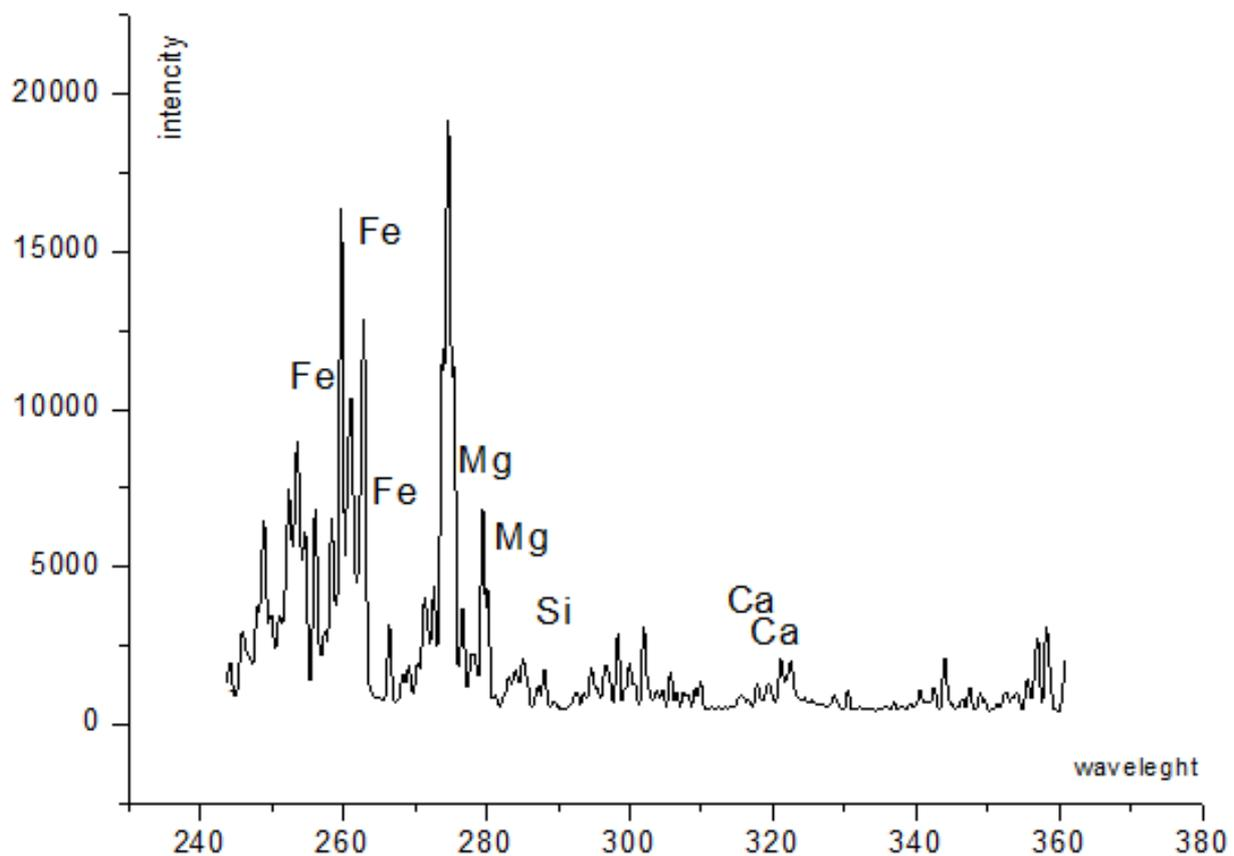
**Pic 2. Typical optical spectrum of unprocessed pelletized iron ore**
