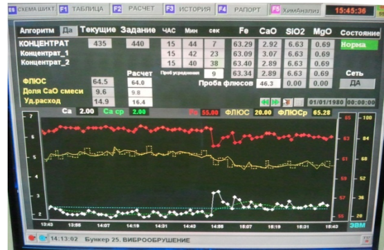
Automated dosage of flux (yellow) as a function of calcium content (white)
